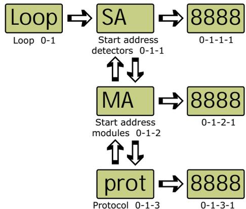
Changing the address of the translator does not entail changing the previously-assigned addresses of the wireless devices, as their new addresses will be assigned automatically (starting from the new address of the translator).
